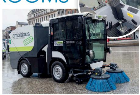
cheap when compared with liquid fuel. "It costs us 75p an hour to power an electric 3.5-tonne sweeper compared with £3.50 to £3.75 an hour to power a diesel," says Smith. And there has been no need for range anxiety, he reports. "They can certainly cope with an eighthour shift," he says.
